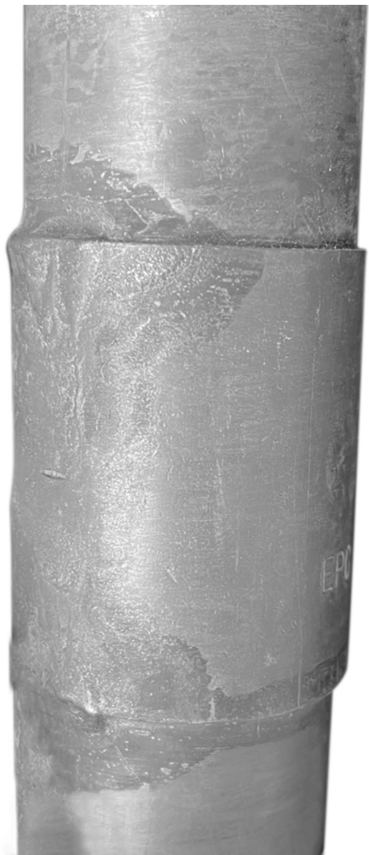
Figure W-434-1 Assembly Partially Brazed Around the Fitting Circumference
