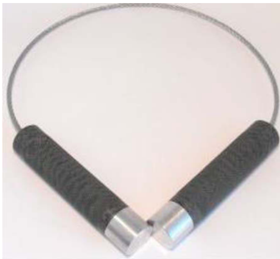
FIG. 1 (b) Permanent Magnet Yoke Method of Part Magnetization (continued)
