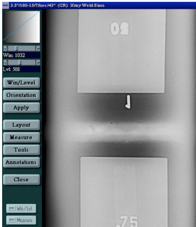
FIG. 26 Pipe Weld Features with Moderate Win-Levels
