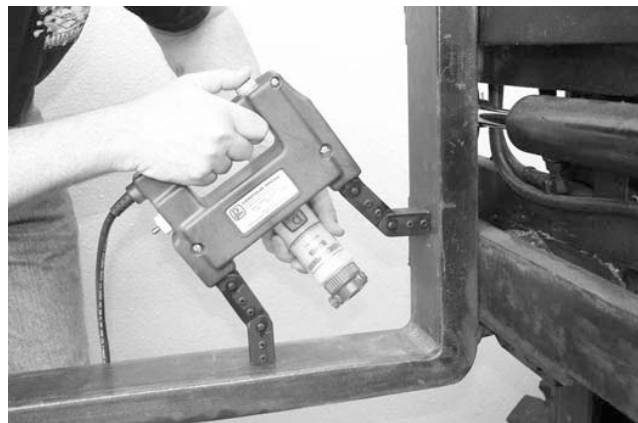
FIG. 1 (a) Articulating Yoke Method of Part Magnetization
