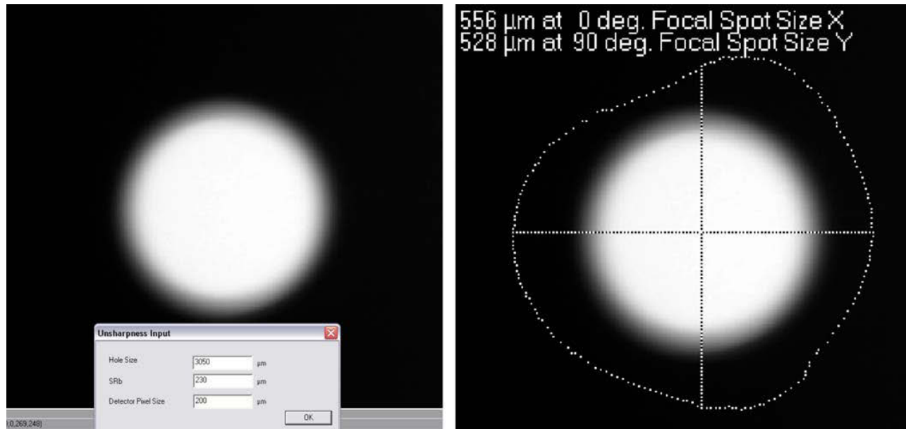
FIG. A1.3 Measurement of the Spot Size of the Four Edges with Threshold from 50 % to 84 % and Extrapolation with Factor 1.4 with Automatic Calculation of the Effective Focal Spot Size in X and Y Direction
