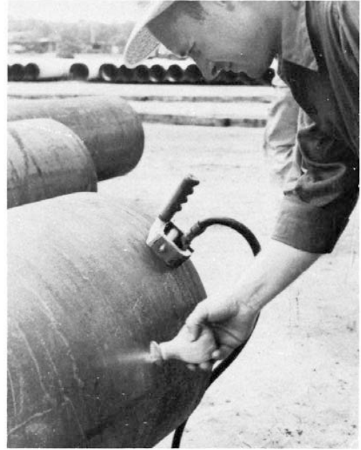
FIG. 5 Direct Contact Magnetization Through Magnetic Leech Clamp of Part
