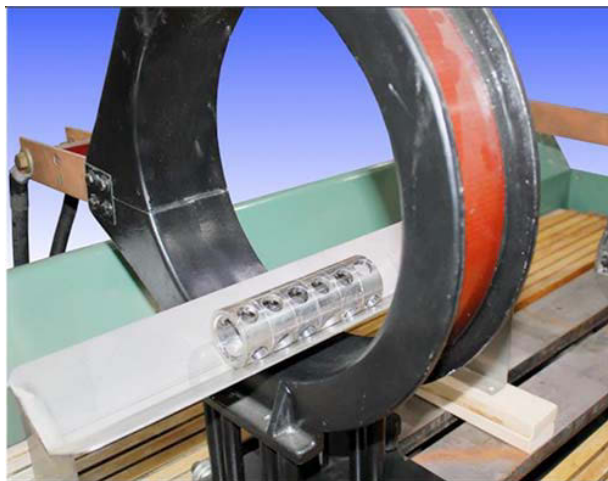
FIG. 11 (a) Magnetic Pole Pieces by Stacking Parts
