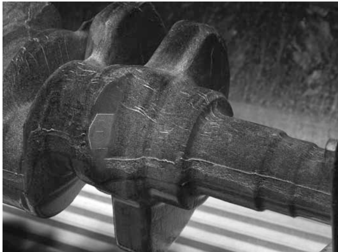
FIG. A1.4 Crankshaft with Various Longitudinal Indications
