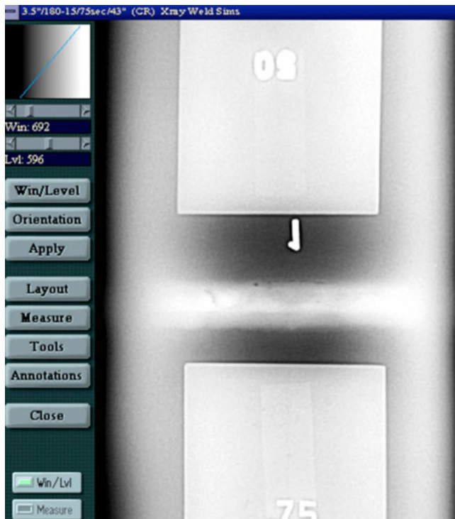
FIG. 27 Pipe Weld Features with Higher Win-Levels
